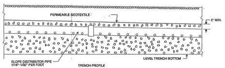
NOTE: DO NOT INSTAULTBENCHES IN WET SOIL INSTALL TRENCHES PARALLEL TO CONTOURS. INSTALL THENCHES AS SHALLOW AS POSSIBLE WHICH MEET ABOVE NOTED MINIMUM DEPTHS. RAKE SIDES AND BOTTOM OF TRENCH PRIOR TO PLACING GRAVEL. ENDS OF ALL DISTRIBUTOR PIPES MUST BE CAPPED
